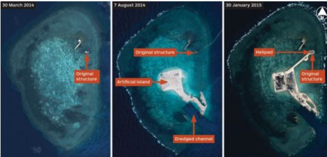
Airbus Defence and Space satellite imagery from 30 March and 7 August 2014 and 30 January 2015 shows the extent of Chinese progress in building an island at Gaven Reefs in the Spratly Islands. By 30 January a pre-existing platform had been joined to the new island and at least one helipad built.
